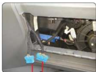
Conector 12 vias Conector 20 vias
